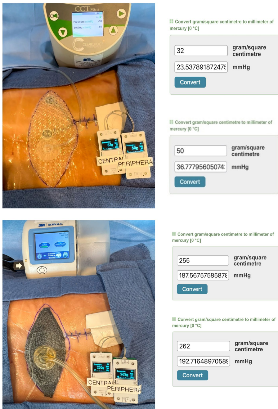
FIGURE 3 | TPE at -50 mmHg and foam at -125 mmHg. Conversion from \text{g}/\text{cm}^2 (on screen) to mmHg shown to the right.
